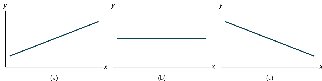
Figure 12.4 Three possible graphs of y = a + bx . (a) If b > 0 , the line slopes upward to the right. (b) If b = 0 , the line is horizontal. (c) If b < 0 , the line slopes downward to the right.
